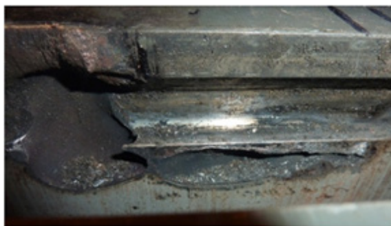
Figure 6. Molten tooth in slot 11
