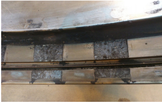
Figure 2. Molten retaining ring fit area
