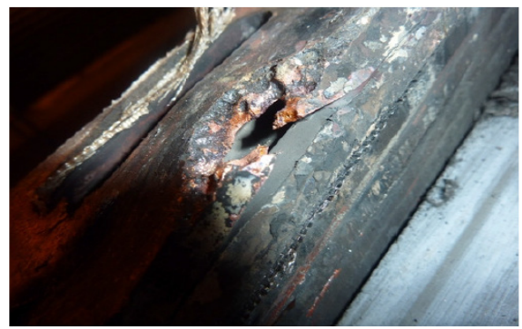
Figure 5. Molten copper from slot 11
