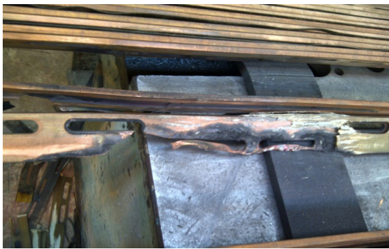
Figure 4. Molten copper from slot 24
